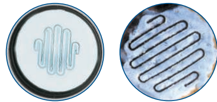
Antibacterial ion membrane after one week (left) and after 8 months (right)
