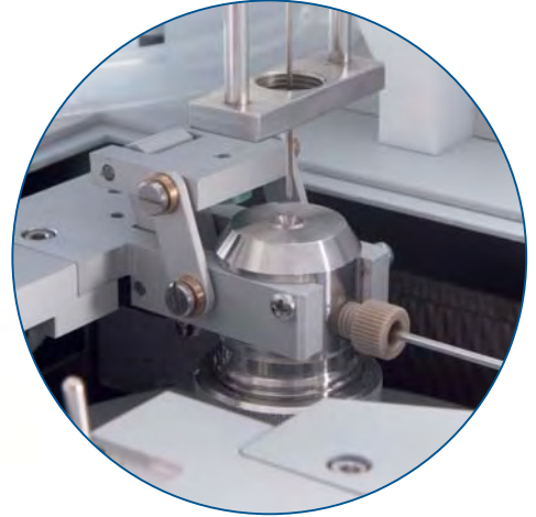
The pneumatic port corresponds to the particle test and conforms with ISO 8254 and DIN EN 1484
